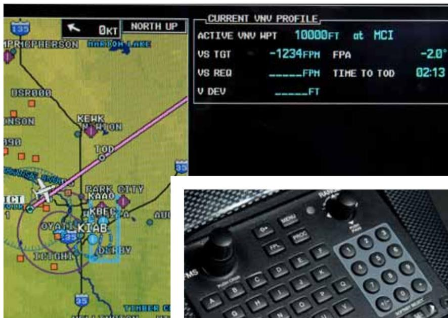
thinking in terms of angles. This causes some confusion, as Garmin systems allow for creating a profile based on vertical speed. However, the system is converting the programmed vertical speed into an angle, based on current groundspeed. This can cause confusion when a pilot tells the system that a 1,500-fpm descent is desired, and then sees that the aircraft actually is descending at 2,000 fpm on the VNAV profile.
