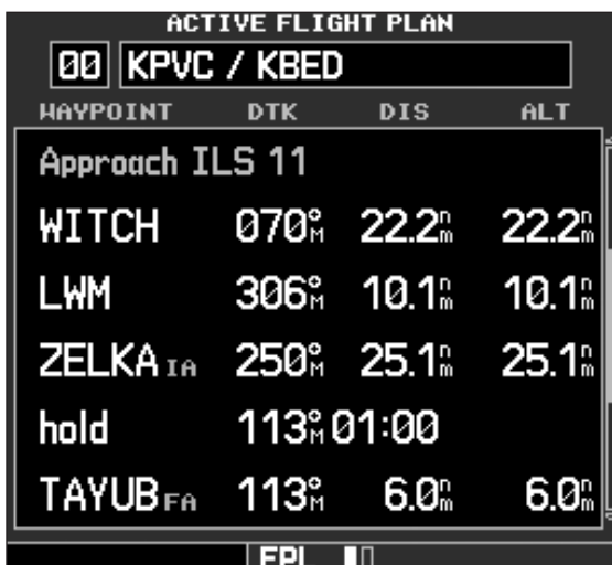
Left: Load the approach into the GPS at the beginning of your brief and do a quick check that paper and screen show the same fixes. This is a good check that you have the right approach in both places and a heads-up if you’ll need to calculate some stepdown that’s not in the database.
